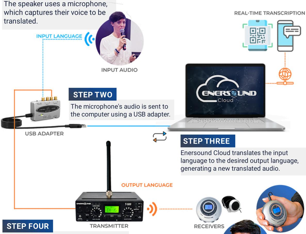
The transmitter receives the translated audio and wirelessly broadcasts it, with a range of up to 500ft.
